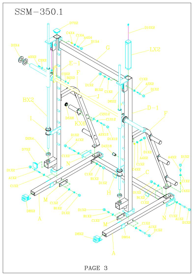
While assembling the smith machine it is very important, that while placing the linear bearing covering the on rod (B). You do so as straight as possible. Failing to do so may cause damage to the linear bearings.
